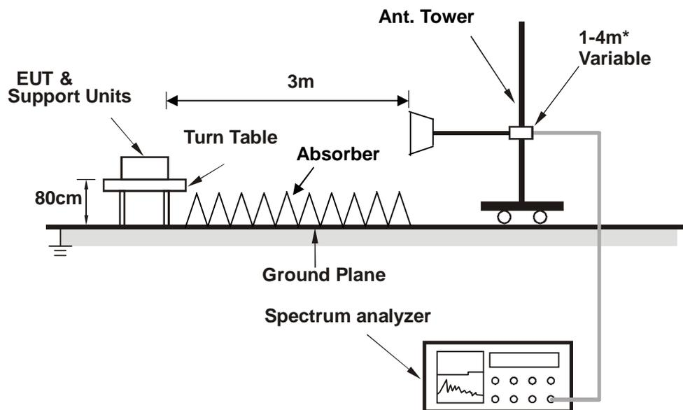
**Note: Cable on the RGP must be insulated.**
